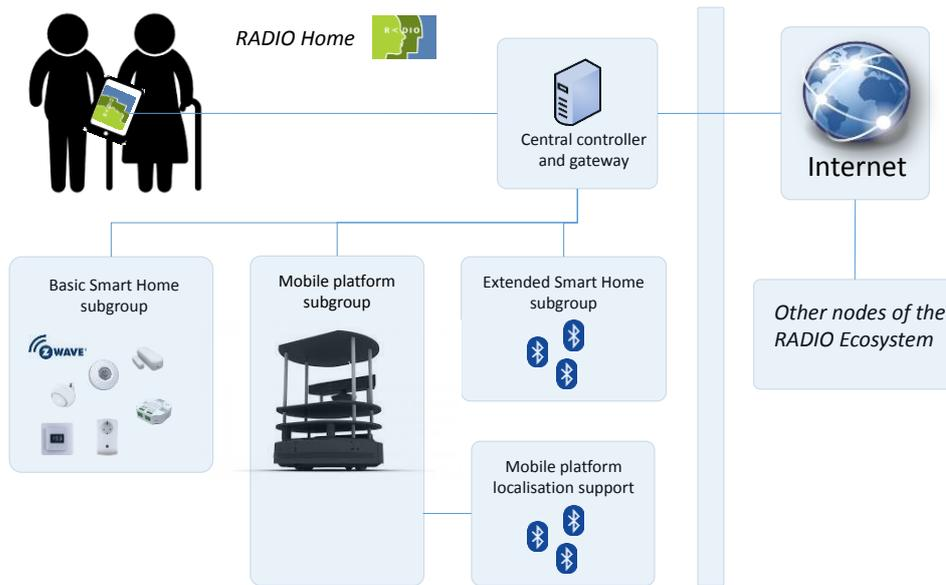
Figure 3: Conceptual architecture of RADIO Home communication channels
