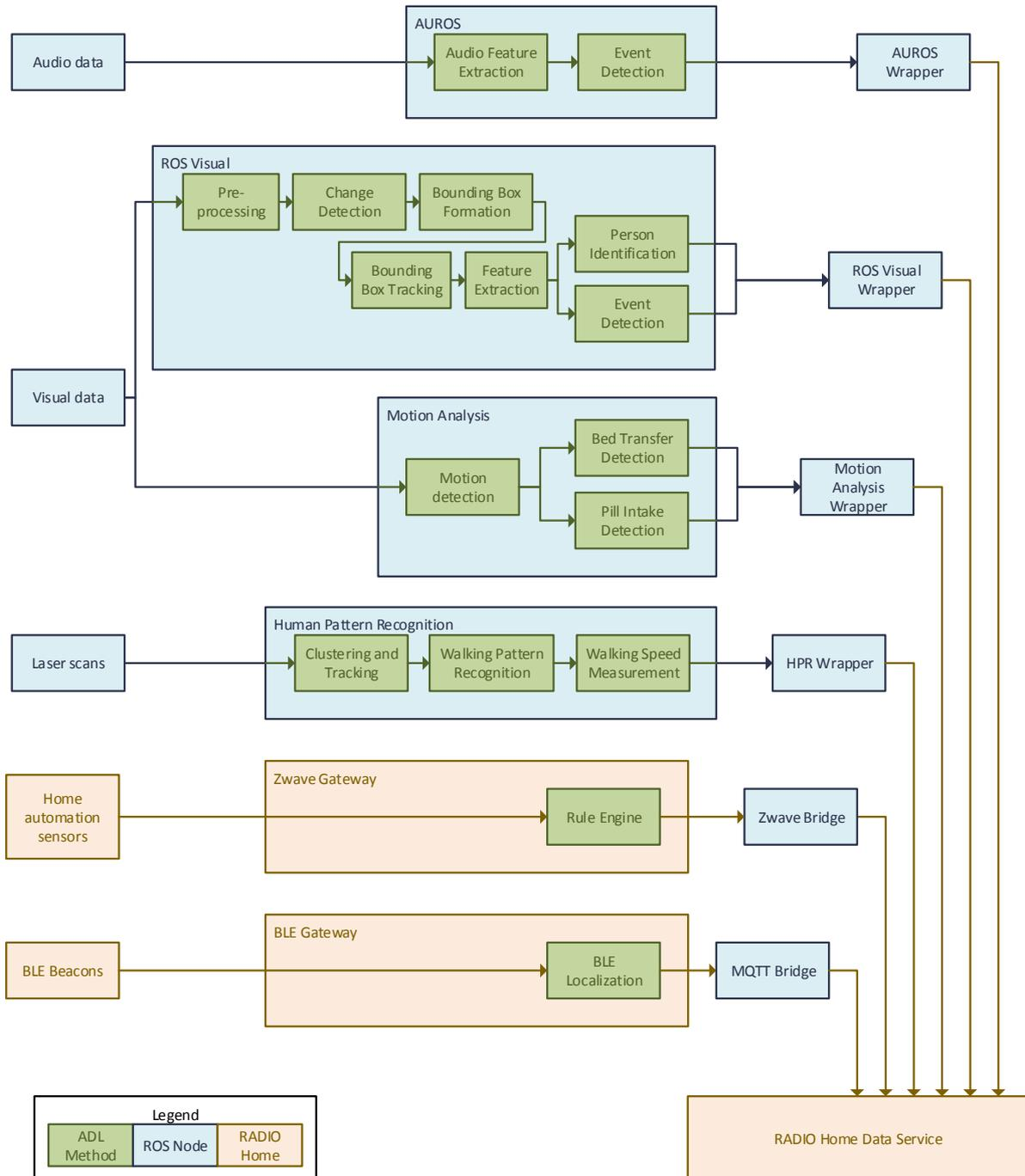
Figure 4: Conceptual architecture of ADL recognition components
