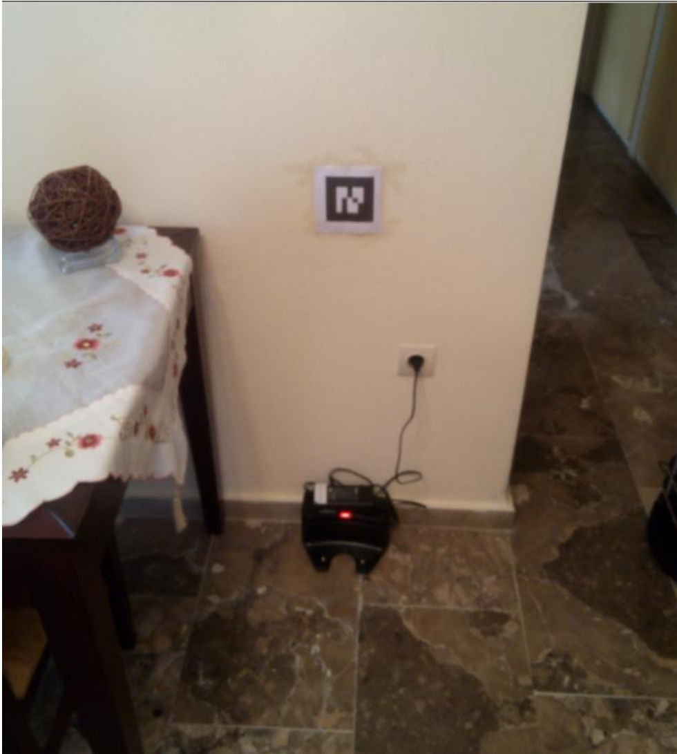
Figure 26. AR code installed above the docking station
