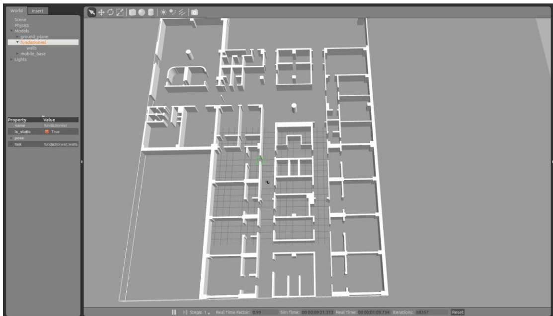
Figure 7: Building conversion for simulation in Gazebo
