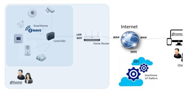
*Figure 2:* enControl<sup>TM</sup> *Service Architecture*
